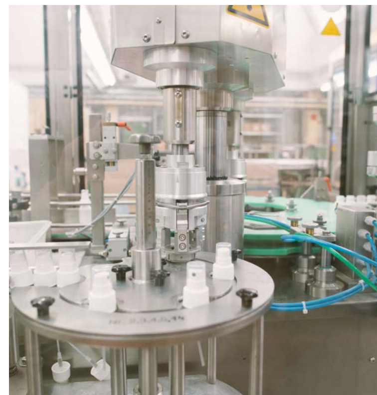
Assembling a pump spray in the bottling process
