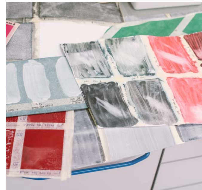
Cleaning tests on different materials in order to check opacity, color application, gloss and more
